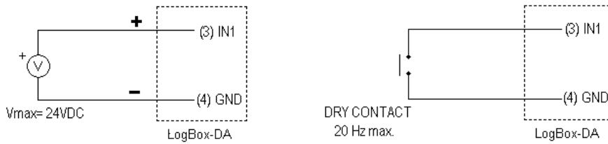
Fig. 10 – Voltage pulse and dry contact channel 1 input
